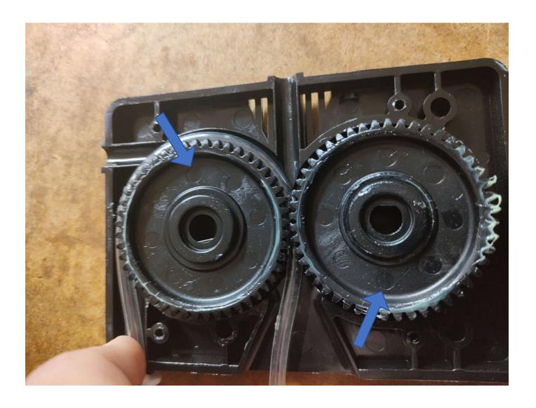
**5.** Close the cartridge and make sure that the tube will not crush between cartridge halves. Test operability by pulling the tube while pressing cartridge halves together.
