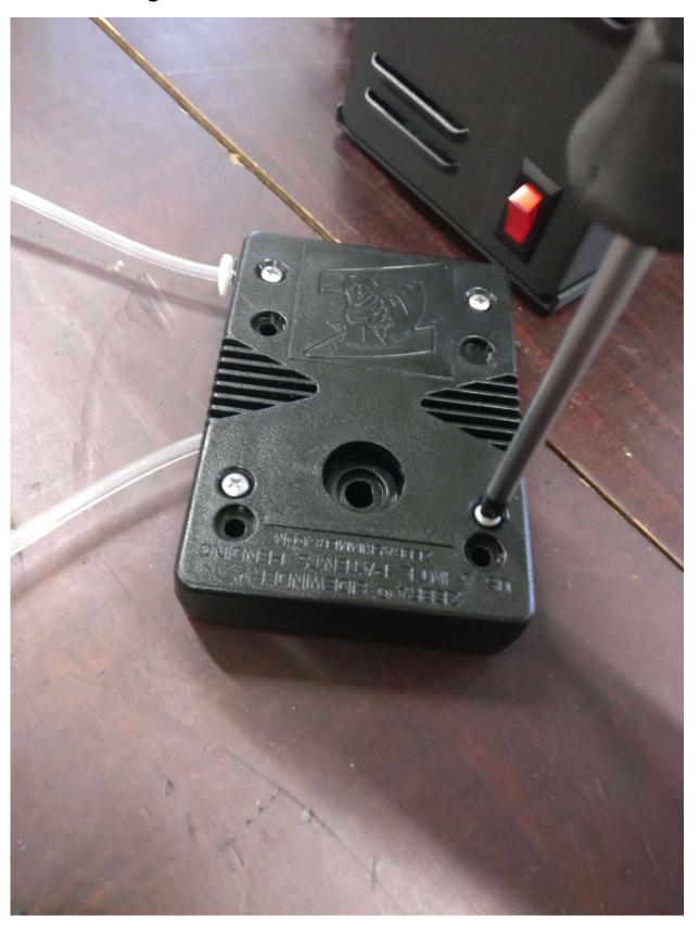
4. Remove the old tube and replace it with new one.
