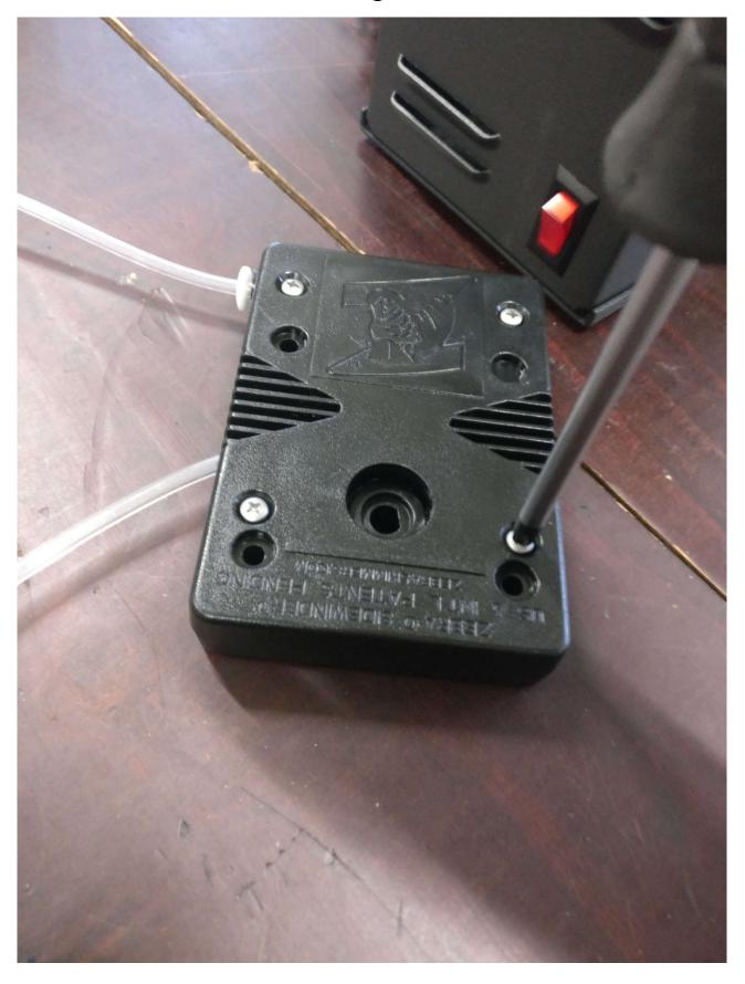
**7.** Assemble cartridge to the axle and twist it to correct position.
