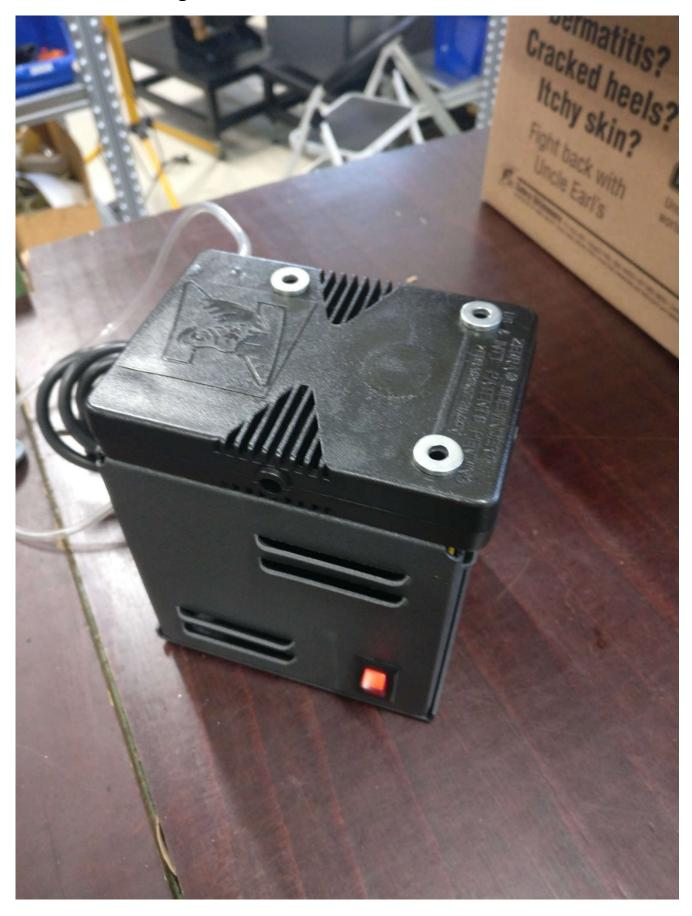
**9.** Assemble the cartridge and the bottom plate with the three screws.
